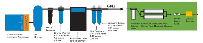
ISO 8573-1 2010: 1, 4, 1 used when ambient temperatures are above 50°F (PFD Diagram Above)
