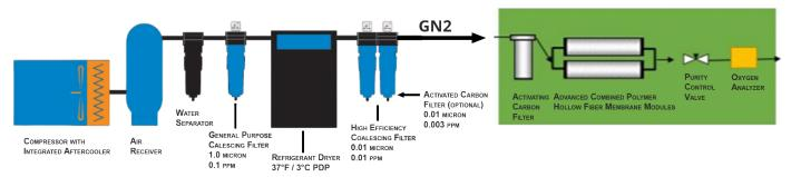
ISO 8573-1 2010: 1, 4, 1 used when ambient temperatures are above  $50^{\circ}F$  (PFD Diagram Above) ISO 8573-1 2010: 1, 2, 1 used when ambient temperatures are below  $50^{\circ}F$
