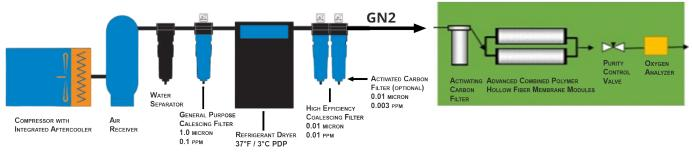
ISO 8573-1 2010: 1, 4, 1 used when ambient temperatures are above 50°F (PFD Diagram Above) ISO 8573-1 2010: 1, 2, 1 used when ambient temperatures are below  $50^{\circ}F$
