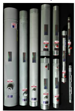
The compressed air, saturated with water vapor flows through a bundle of **GENRON®** hollow-fibers. The membrane fibers allow water vapor to pass. The air stays in the membrane fibers and is discharged as dry product. A fraction of the dry air is redirected internally to sweep the permeated water vapor as a gas out of the module.
